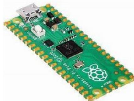
Fig 4.5: Raspberry Pi Pico Board
