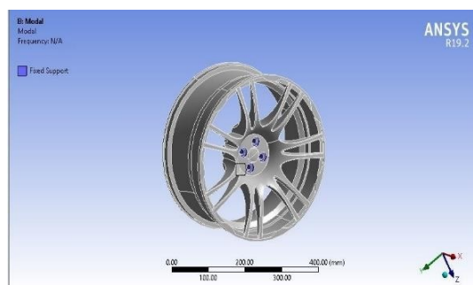
Fig:6.1 Wheel studs fixed at center plain axis
