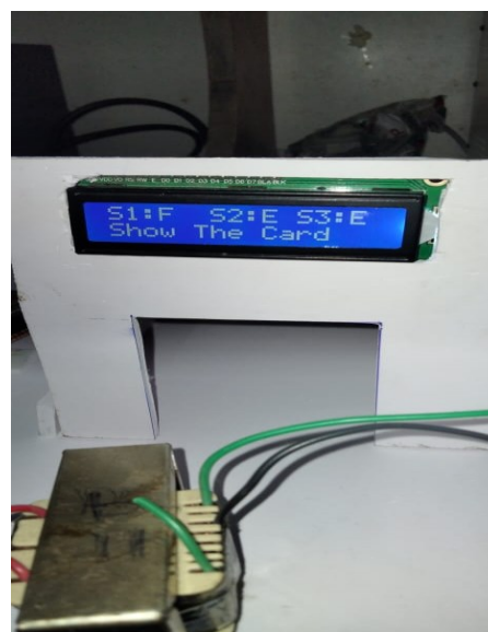
Figure.8 Slot status on LCD
