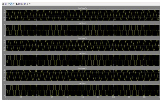
Fig. 8: 3-Phase voltage & current wave forms of Load, Grid
