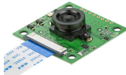
Fig-3: Raspberry pi Sony 8mp camera
