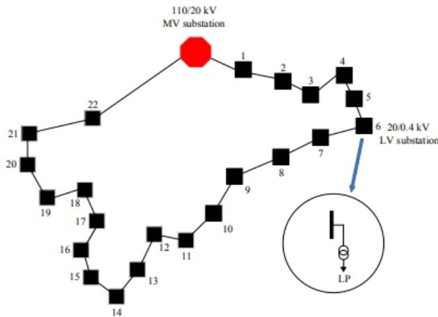
Fig. 2. Single line diagram of the test system
