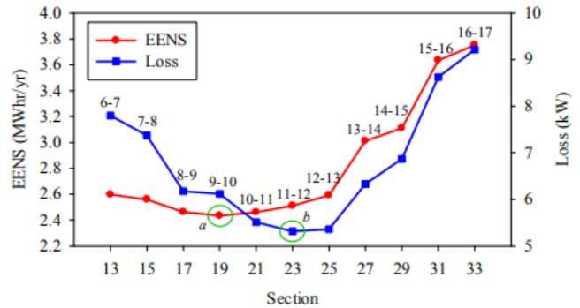
Fig. 3. EENS and Loss in various NO switch locations
