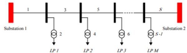
Fig. 1. A typical loop-structured distribution network
