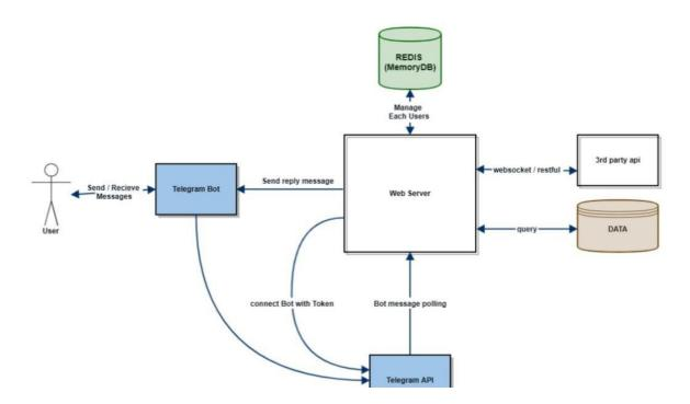
The architecture of the Telegram bot is built on a client-server model, where the client (user) interacts with the bot, and the server processes and responds to commands. The main components include:
