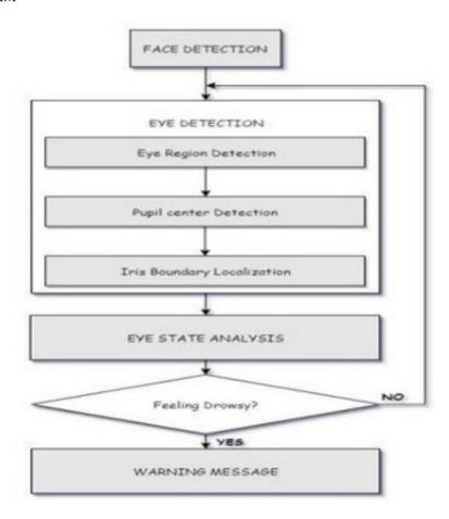
The system will be continuously monitoring the movement of the driver's eye by a live camera and all the monitored signals are pre - processed. A Black Boxwiththesoftwareinstalledisusedto detect the driverdrowsiness and alertsthe driver withbuzzer, if driver is affected by drowsiness.
