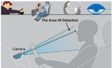
The value we will use to determine how long the person has closed his eyes is threshold value. So if both eyes are closed, we will keep on increasing score and when eyes are
