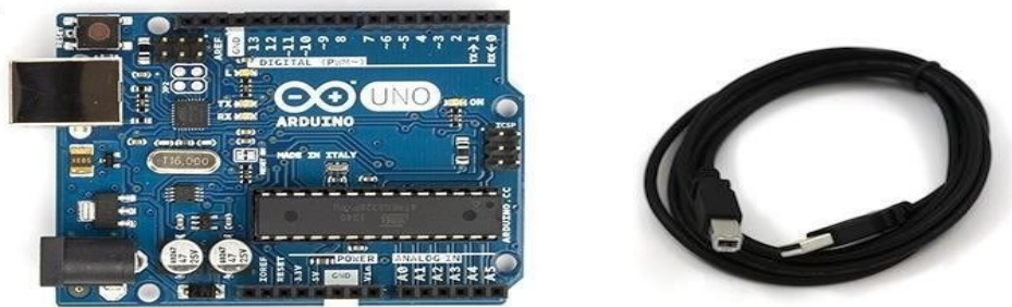
Fig. 4 Arduino board and USB cable
