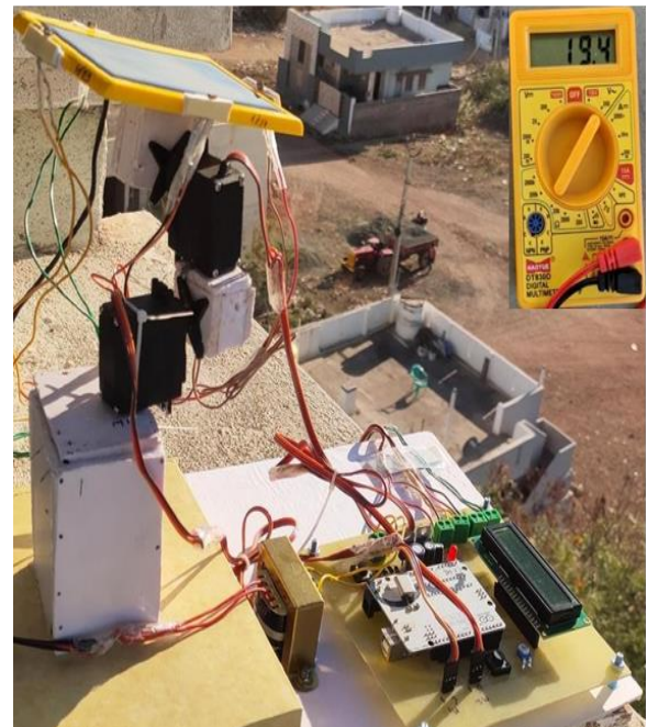
Fig 7 when LDR3 has more light intensity
