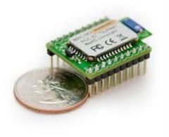
Bluetooth is an open wireless technology standard for exchanging data over short distances (using short wavelength radio transmissions) from fixed and mobile devices, creating personal area networks (PANs) with high levels of security. Created by telecoms vendor Ericsson in 1994 it was originally conceived as a wireless alternative to RS-232 data cables. It can connect several devices, overcoming problems of synchronization.
