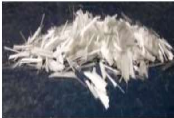
Fig.4.1. Glass Fibres used.
