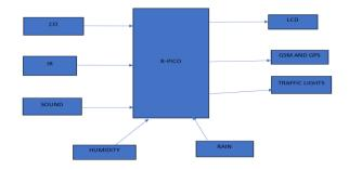
In the proposed traffic management system, the integration of Raspberry Pi serves as a central component to revolutionize the way urban mobility is regulated. The system envisions the deployment of Raspberry Pibased devices equipped with an array of sensors to remotely monitor real-time weather parameters and pollutants. These sensors would include weather sensors to capture data on factors such as temperature, precipitation, and visibility, as well as pollutant monitoring sensors to assess air
