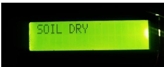
Figure 6: Output of Soil Moisture sensor
