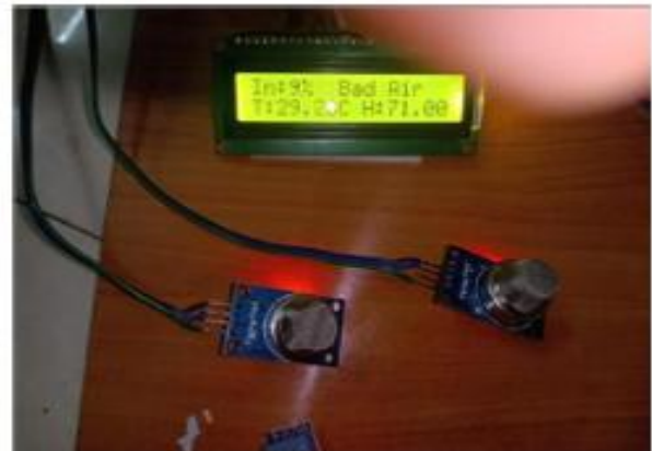
Fig 5.4 LCD Display showing Bad Air quality.
