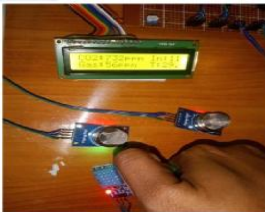
Fig 5.3 LCD Display showing PPM values.
