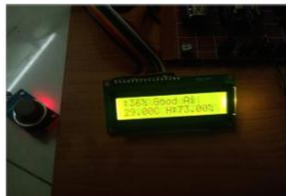
Fig 5.1 LCD Display showing Good Air Quality
