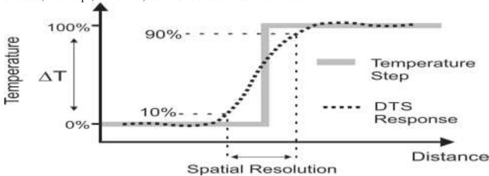
Fig. 1. Example of DTS spatial resolution defined by temperature step.
