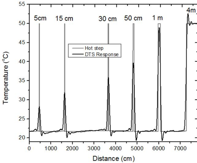
Fig. 2. Experimental results used to identify the DTS system model.
