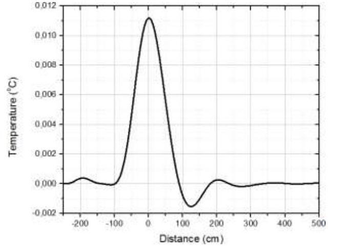
Fig. 4. Estimated DTS system impulse response  $h(z)$ .
