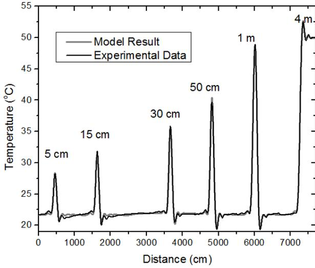
Fig. 3. Experimental results vs. estimated DTS model.
