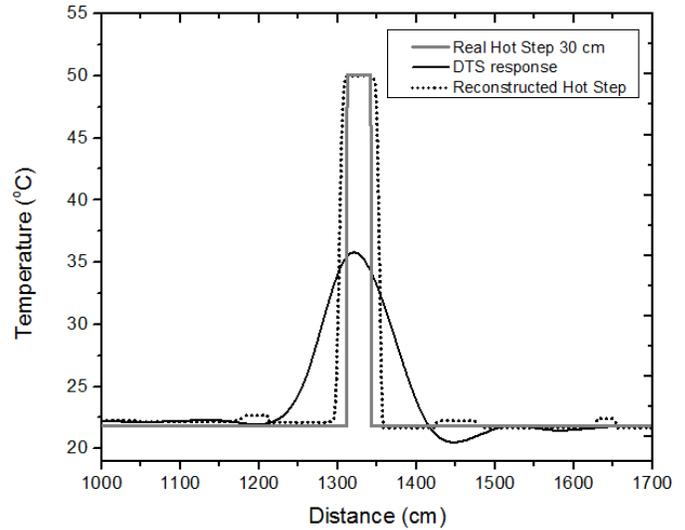
Fig. 7. Result of hot step reconstruction with 30 cm length and 50 °C.
