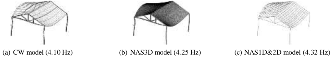
Fig. 23 Third modal shape of the industrial building.
