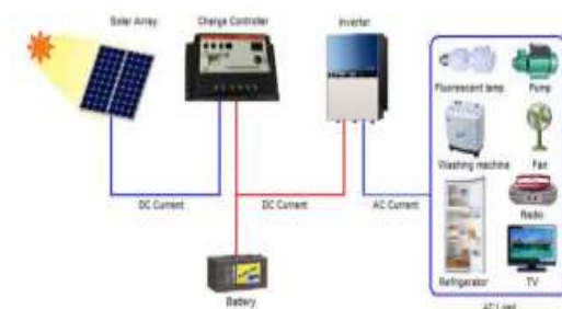
Figure 1. Schematic diagram of a typical "Solar Home System."
