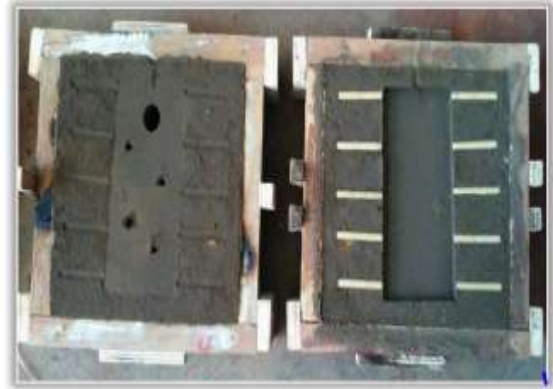
Figure 1: Sand mould with chills
