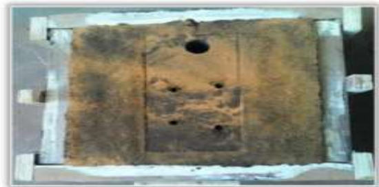
Figure 1: Sand mould with chills
