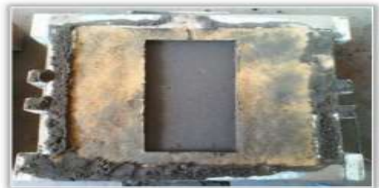
Figure 2: Sand mould without chill Table 1: chemical composition of the cast aluminium alloy
