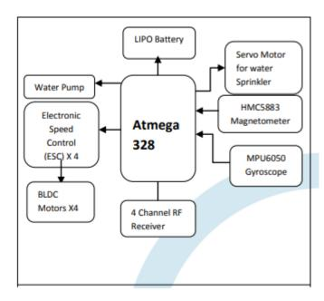
Fig. 1 Block diagram of Agriculture Drone.
