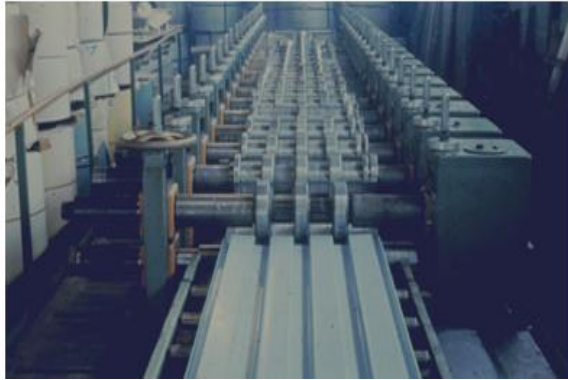
Figure 2: Image showing Rolled Formed Operation Un-stiffened Element
