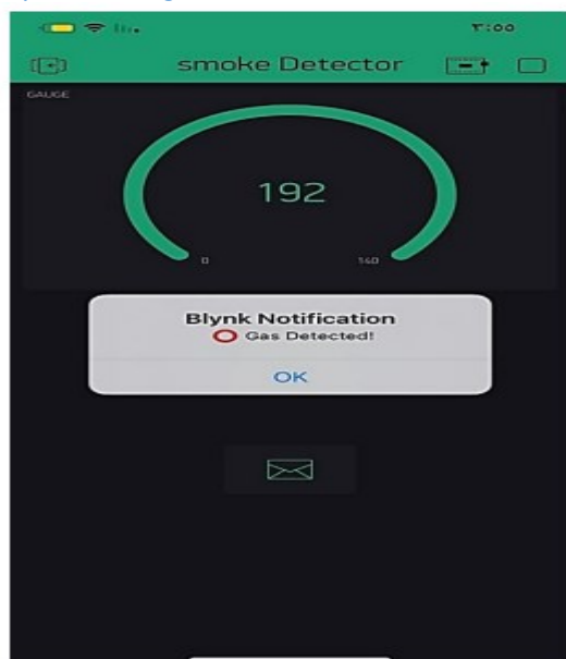
Fig. 6: Blynk app notification for gas leakage case.
